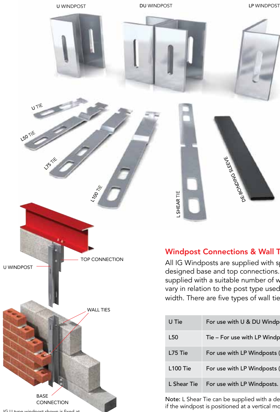
IG U type windpost shown is fixed at the base to concrete and at the top to the underside of a steel beam.
